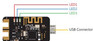
Power: Input voltage 2S~7S LiPo battery (6-30V)
